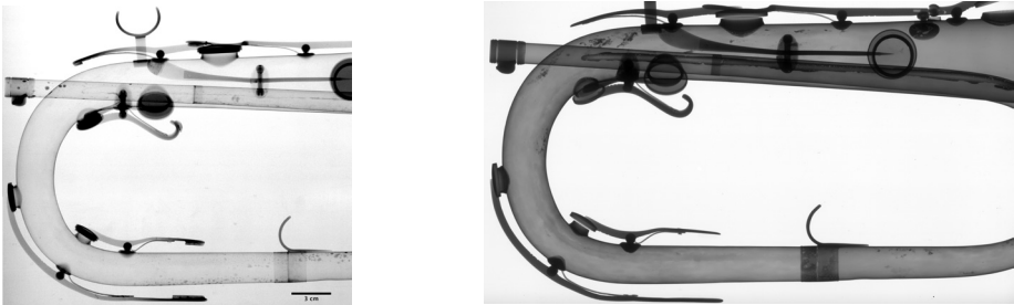
Figure 11: Neutron (left) and X-ray (right) radiographs for the Müller keyed bugle (Appendix, no. 20; for an overview of the chemical composition, see Figure 1).
